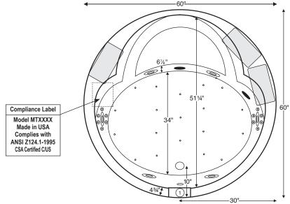
Numbered area on tub deck represent possible location to install a cleaning system, faucet or other fixtures. Note: A hand shower or Breda valve may be located on the tub flange above any of the four jets on the sides of the tub. Shown with Air Massage and Ultra Whirlpool Package.
